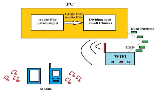
Figure 2.System Architecture
