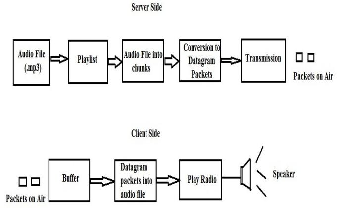
Figure 1.Components of Campus Radio
