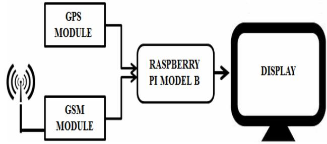
Fig. 9. Client side system block diagram.
