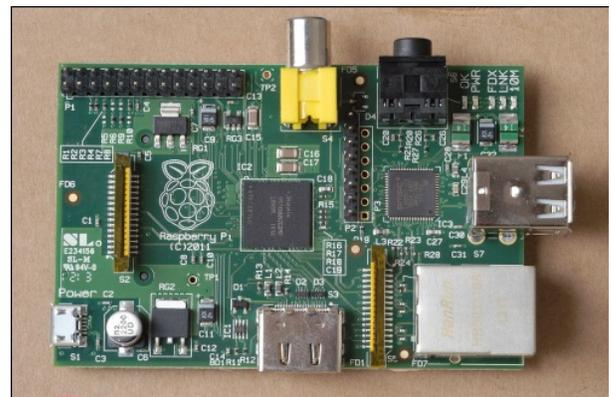
Fig. 3. Raspberry Pi model B
