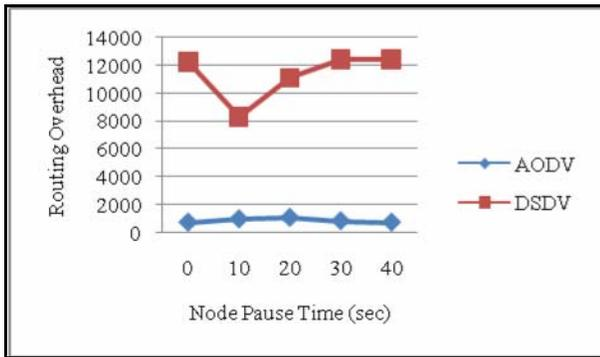
Figure 12. Impact of the node's pause time on the routing overhead
