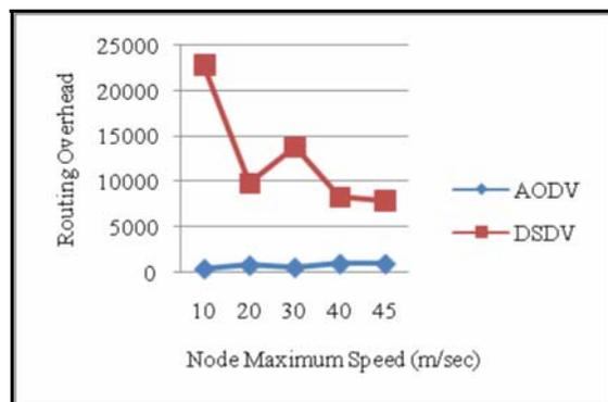
Figure 6. Impact of the node's maximum speed on the routing overhead
