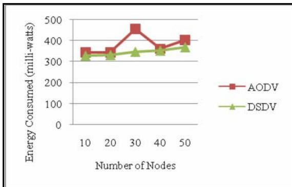
Figure 4: Impact of network size on the energy consumption
