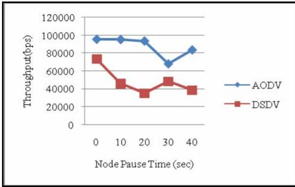
Figure 11. Impact of the node's pause time on the network throughput
