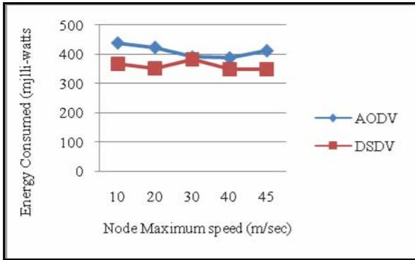
Figure 7. Impact of the node’s maximum speed on the energy consumption
