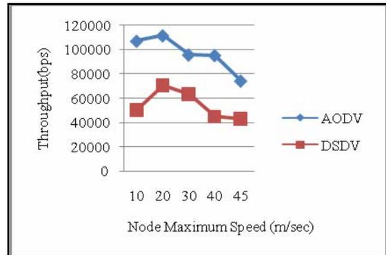
Figure 5. Impact of the node's maximum speed on the network throughput
