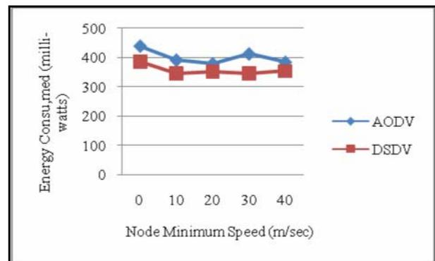
Figure 10. Impact of the node’s minimum speed on energy consumption
