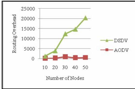
Figure 3. Impact of network size on the routing overhead
