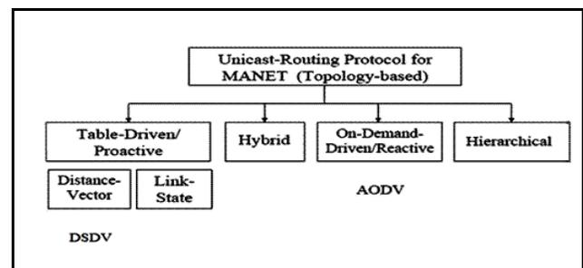
Figure1. Classification of routing protocols in MANET
