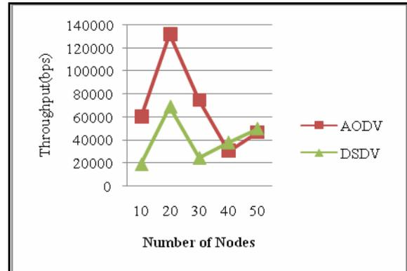
Figure 2. Impact of network size on the throughput
