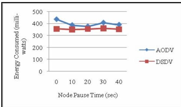
Figure 13. Impact of the node's pause time on energy consumption
