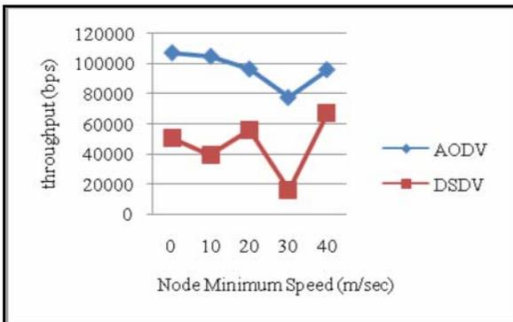
Figure 8. Impact of the node’s minimum speed on the network throughput
