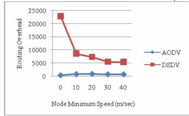
Figure 9. Impact of the node’s minimum speed on the routing overhead
