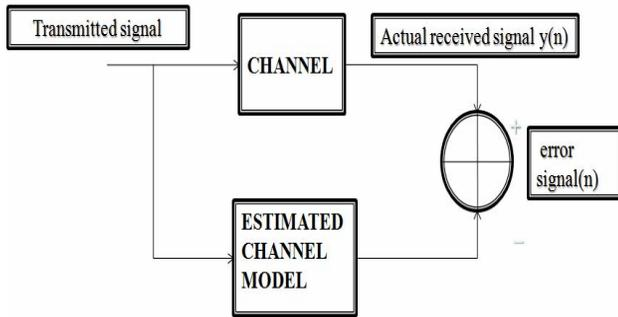
Figure 2. Channel estimation Model
