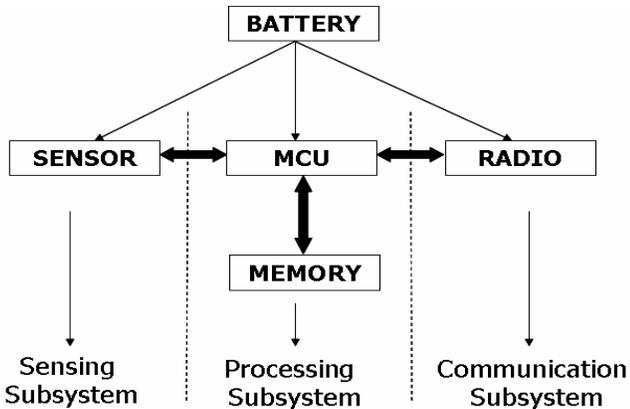
Figure 1. Architecture of a typical wireless sensor node
