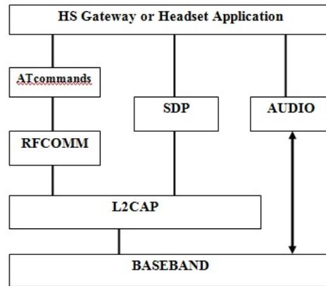
Fig. 2 : Configuration of Protocol Stack for Headset Model Usage
