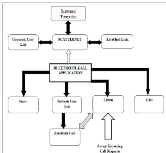
Fig. 4: Block Diagram of “Voice Call Implementation Using Bluetooth Scatternet”
