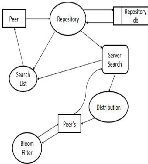
Figure4. Data Flow in P2P Network with Repository Function
