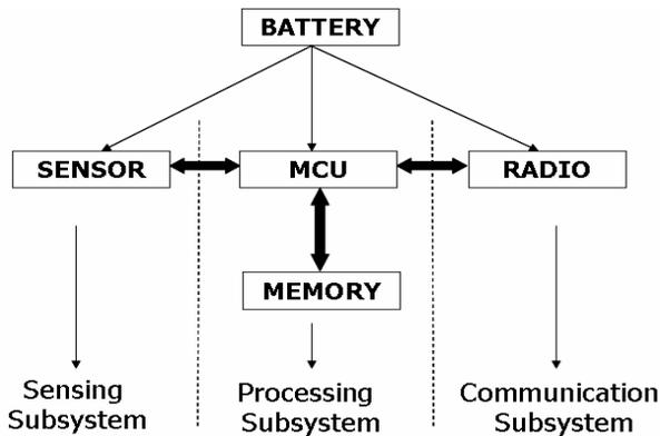
Figure 1. Architecture of a typical wireless sensor node
