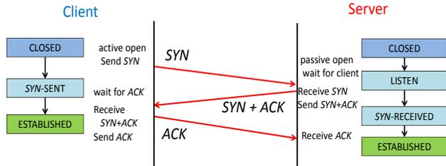
Fig 1. TCP Three-way handshake
